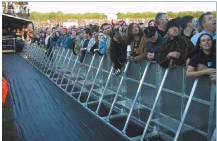
Figure 37 Front-of-stage barrier used at right-angles to the stage
